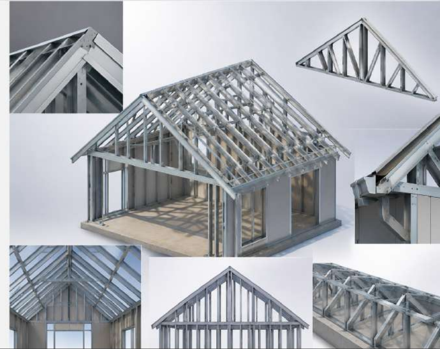
PITCHED ROOF - TYPICAL CFS RAFTER / TRUSS CONCEPT
