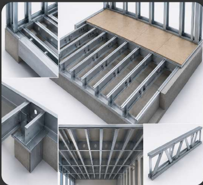
TYPICAL CFS FLOOR / JOIST ASSEMBLY
